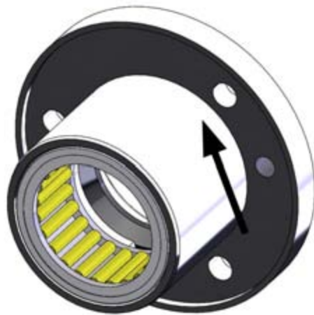
Figure 34. Spreading area of the adhesive compound
