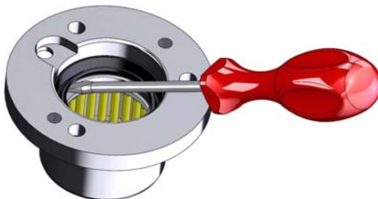
Figure 29. Removing the rear bearing seals
