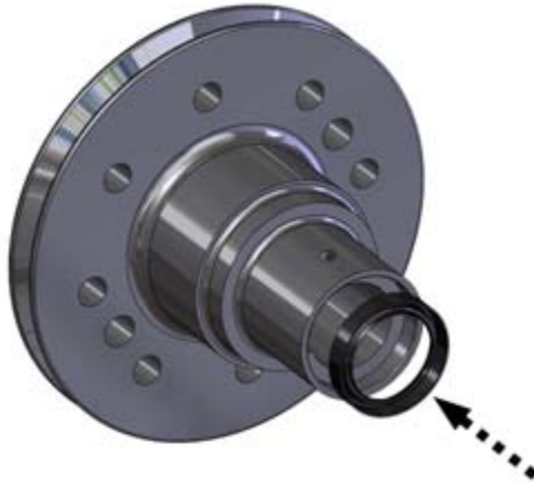
Figure 21. Installing the coupling flange shaft seal
