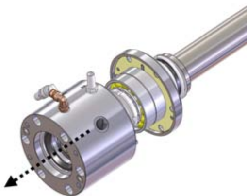
Figure 6. Bearing housing, shaft, bearings, and mechanical seal
